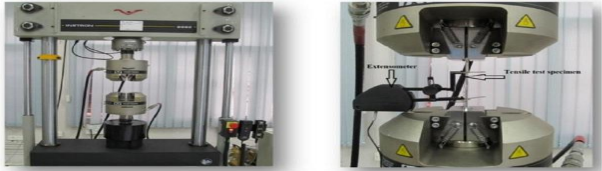
Fig. 7 (a) Universal Testing Machine (INSTRON) (b) Specimen mounted over UTM along with extensometer
